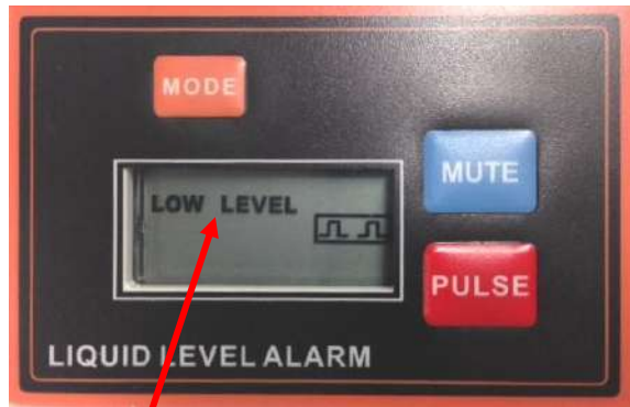
LOW LEVEL alarm mode displayed.
